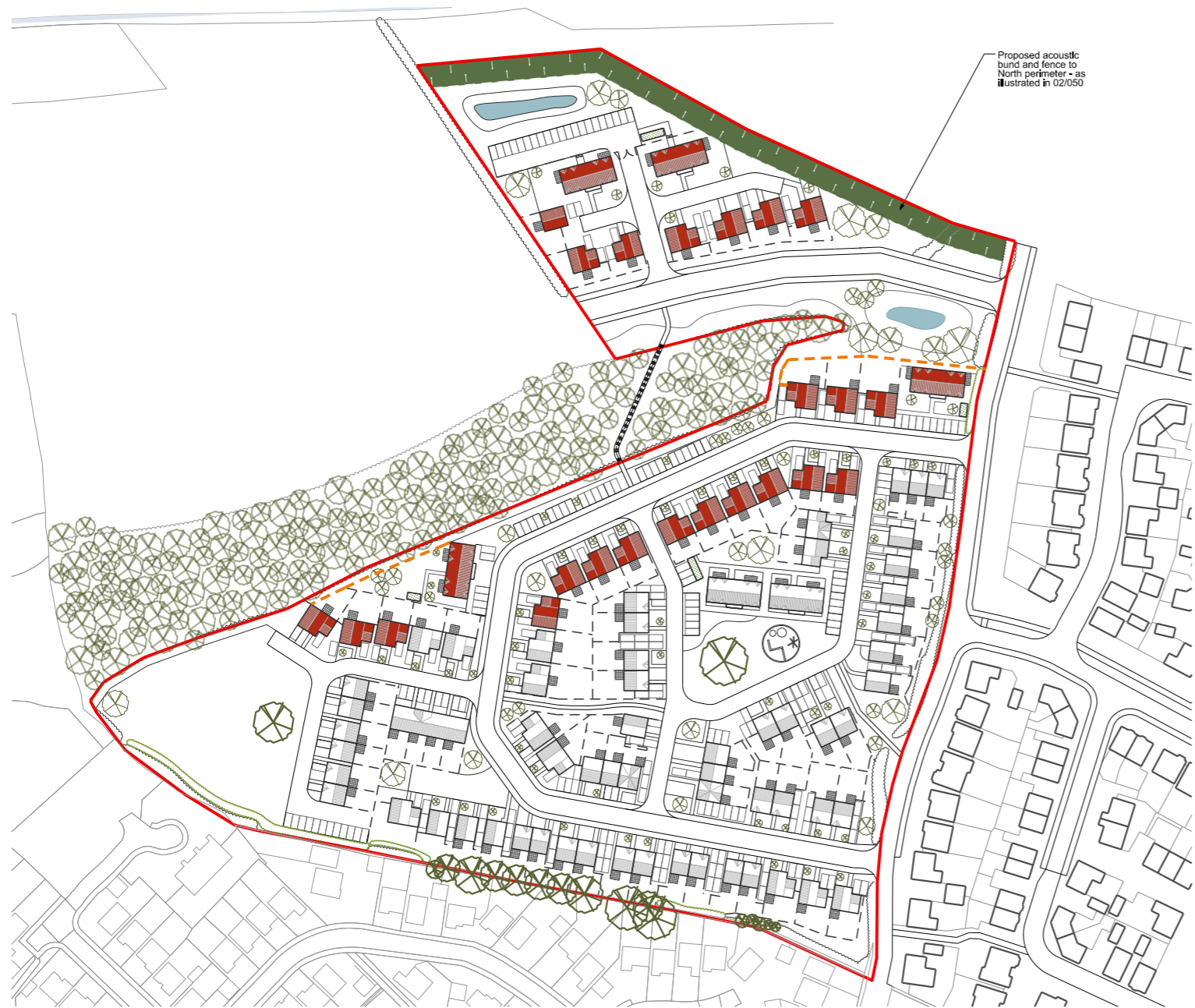
01 PROPOSED SITE PLAN - NOISE MITIGATION STRATEGY 050 SCALE:- 1:1000 @ A3
