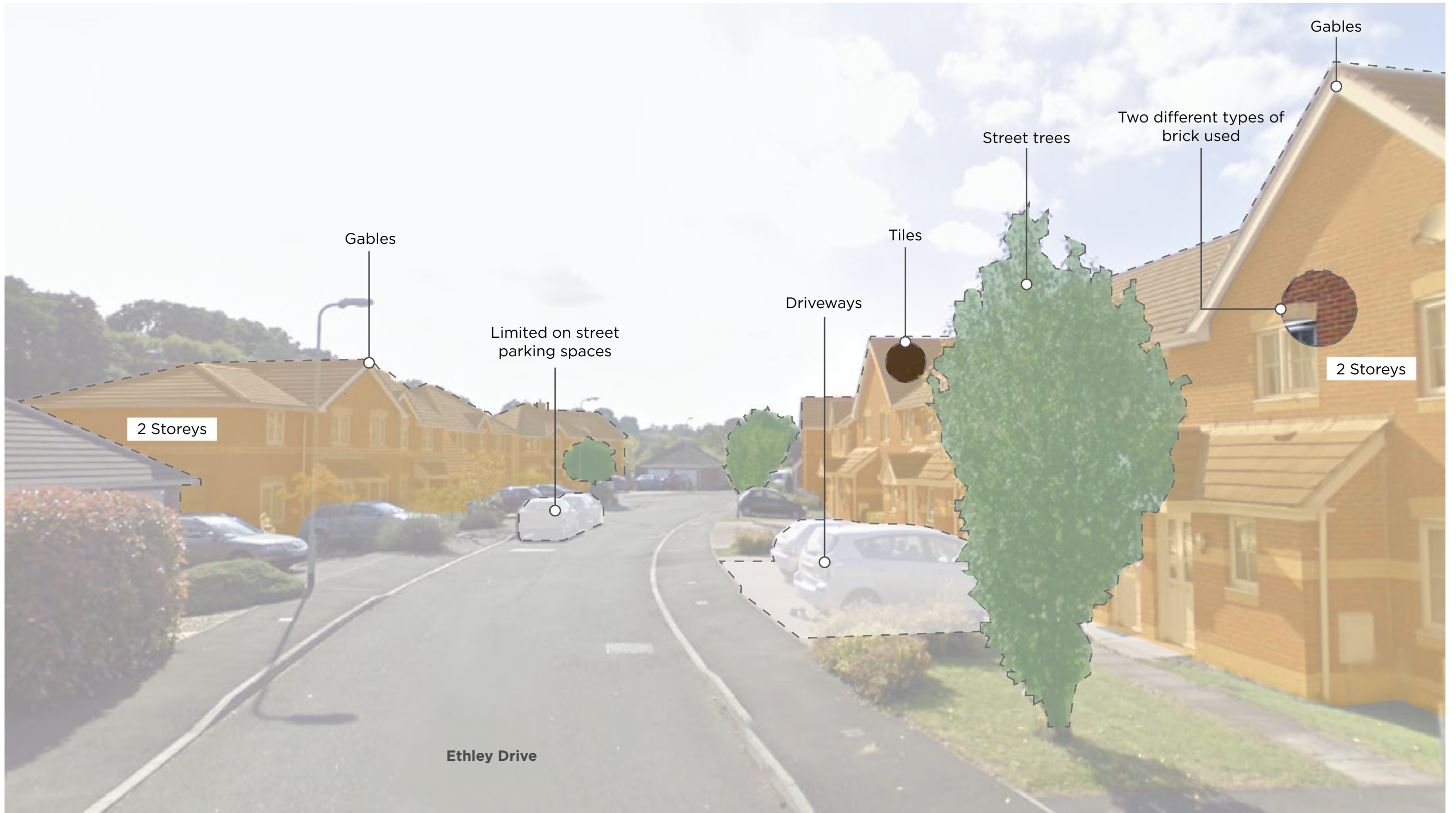
Consistency in building form, heights and material helps to create a more unified street scene along Ethley Drive
